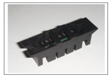
The 16036503 Calpak uses part number 16036504 for the resistor network, the former part number being the actual assembly in a carrier. The chip itself has been produced in two different packages: A plastic DIP package and a ceramic DIP package. The chip uses a series of printed carbon elements that are laser-trimmed to achieve given precision resistance values. The carbon resistance pads are printed on both the top and the bottom of the ceramic substrate.
