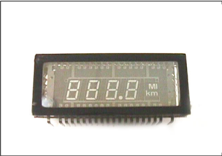
Fractured VFD display. Note the white spot in lower left corner.
