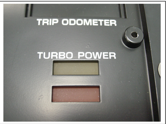
Regal with turbo engine option. Turbo boost indicators for low and high boost display.
