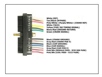
And this is the 1986-1987 CCCI. Note the difference in Crank Signal and Crank Ground colors:
