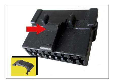
This latch keeps the connector properly aligned in the dash cradle, allowing the electrical connections to engage with the angled PC board attached to the digital portion of your cluster. Without the latch in place, the connector will "float" behind the digital assembly, mis-aligning the connector with the mating part.
