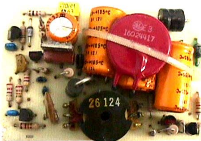
Early power supply board using external RF choke remotely mounted.
